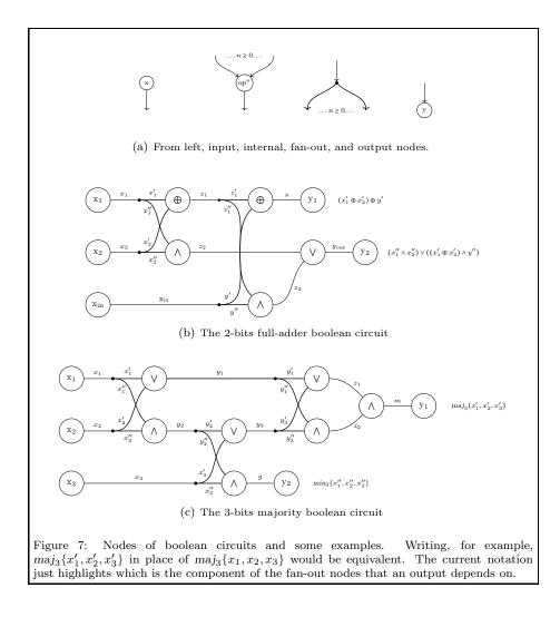
complexity classes such as NC, AC, and  $P/_{poly}$ . The contribution of this work to these encodings is in the use of copy and discard to directly express the fanout nodes that allow a more compact and modular representation of circuits. In particular, as compared to [26, 18, 2], our encoding is able to get rid of the garbage that accumulates in the course of the simulation.
