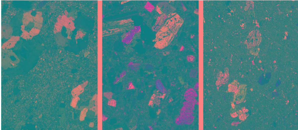
Fig. 1. Photomicrographs in cross-polarised light of samples MNS-01 (left), MRL-03 (centre) and OLV-01 (right), taken at same magnification (field size: 9.71 x 13.07 mm). Anomalous interference colours of crystals are due to section thickness of 45 \mu\text{m} . 82x35mm (600 x 600 DPI)
