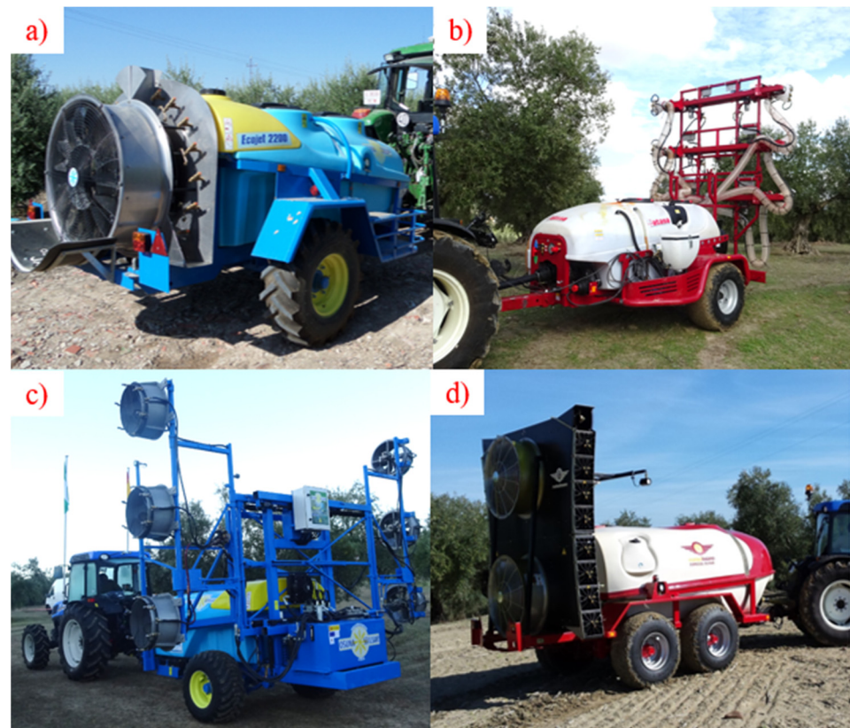
Figure 3. Sprayers used in the trial: (a) Conventional air blast sprayer; (b) P1 prototype; (c) P2 prototype and (d) P3 prototype.
