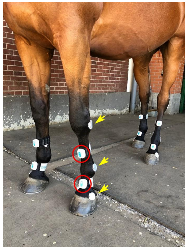
Figure 1. Placement of IMUs (red circle, identified only in one limb) and optical markers (yellow arrows, OMC technology) on equine distal limbs for data acquisition. The IMUs were fixed to the dorsal metacarpus/metatarsus and to the dorsal aspect of the pastern in the four limbs by means of plastic docking bases attached to elastic bands. Optical markers were glued to the skin on the lateral aspect of the joints studied.
