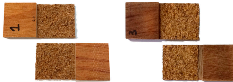
Figure 3. Total (100%) cohesive failure of the cork core (0% wood failure) on specimens tested after dry conditioning ( left ) and immersion in boiling water ( right ). The numbers 1 and 3 on the specimens are testing codes referring to the panels from which they were cut.
