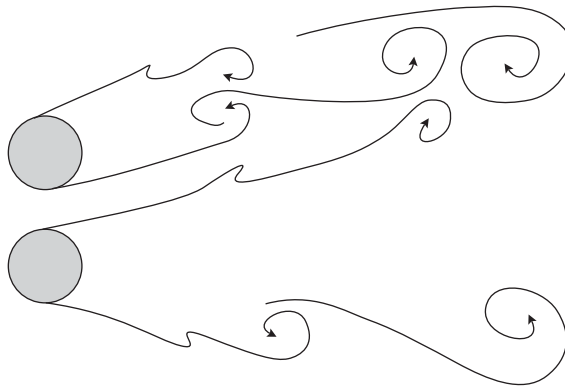
FIGURE 1. Sketch of the biased gap flow pattern and related vortex dynamics characterizing the near wake of two side-by-side cylinders during the flip-flopping regime.
