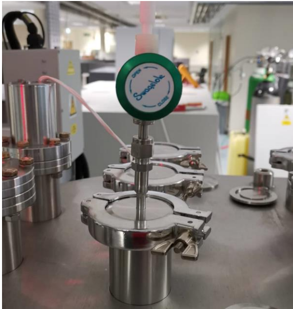
Figure 3-21: Swagelok valve to control the leak.
