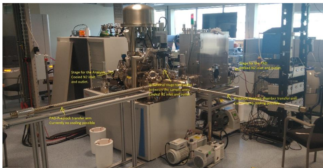
Figure 3-4: A photo for the XPS-PAD system including two transfer arms between them and three cooling stages.
