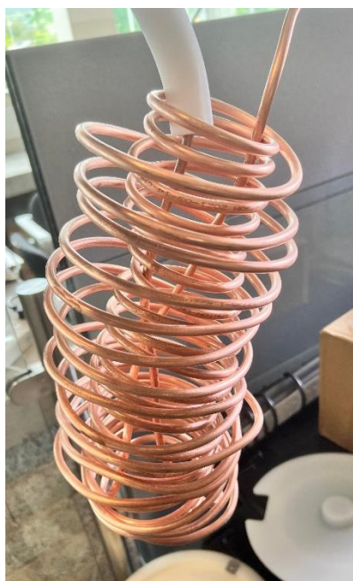
Figure 3-9: A handmade custom-design double helical coil with 50 turns.
