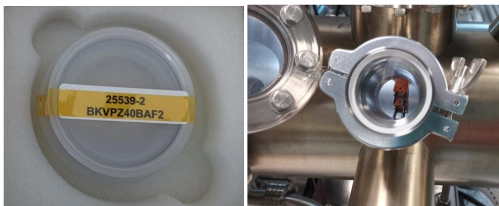
Figure 3-25: A trial of measuring the temperature inside the preplock using IR probe and BAF2 transparent window.
