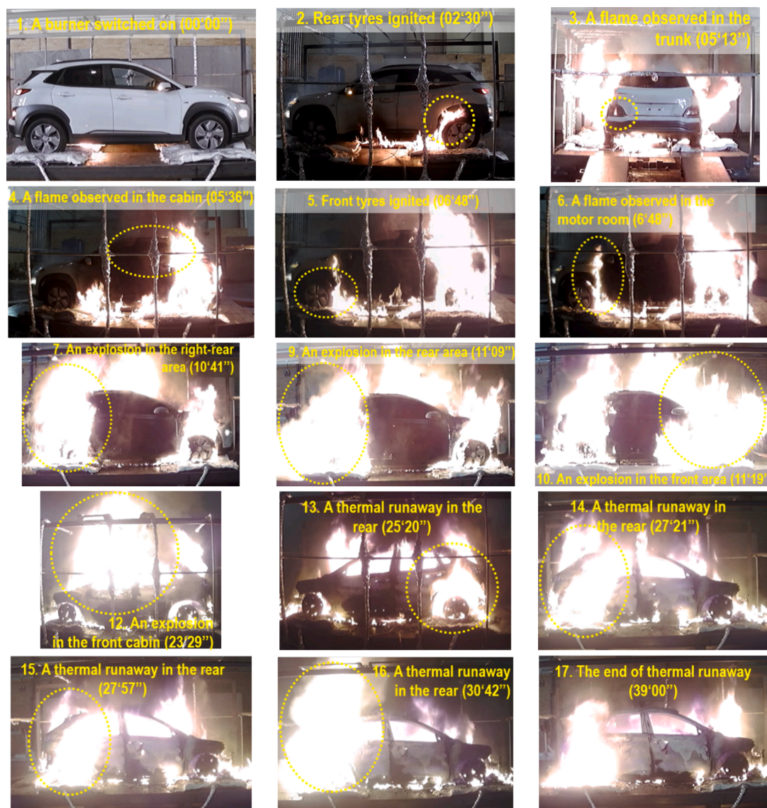
Fig. A1. Photos of the specimen status at the critical events in Test 3.
