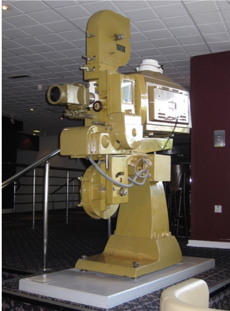
Figure 29: A Gaumont-Kalee GK21 35mm cinema projector. From the collection of The Science Museum Group on display in the café of the PictureVille Cinema at The National Science and Media Museum, Bradford, UK.
