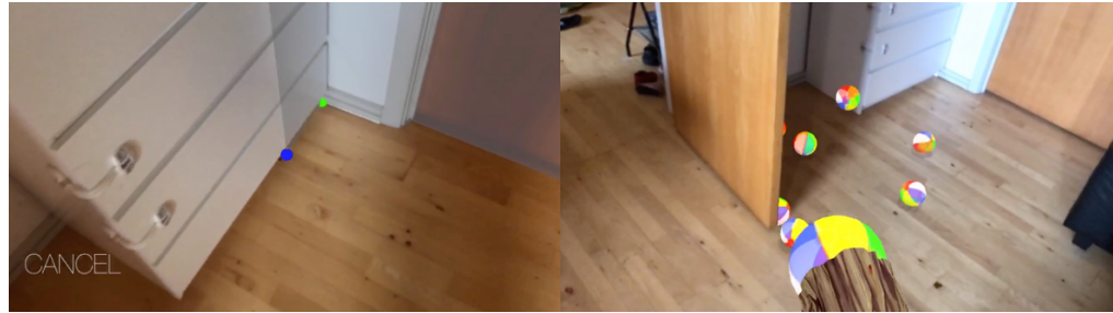
Figure 37. Plotting vertical planes to define real-world geometry. (left). Using the defined geometry to enable virtual content to seemingly occlude and interact with the real-world in a virtual ball-shooting AR game (Lundgren, 2017).
