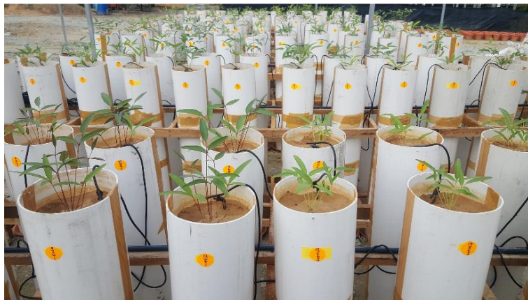
Figure 4-1 (A) Schematic representation of soil-filled PVC column of 20 × 110cm (inside diameter and length, respectively), placed on a perforated plate (B) PVC column setup under rainout shelter including a wooden frame for structural support and (C) column split and root washing.
