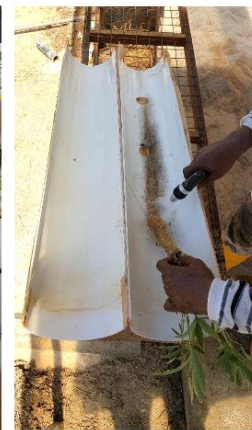
Figure 4-1 (A) Schematic representation of soil-filled PVC column of 20 × 110cm (inside diameter and length, respectively), placed on a perforated plate (B) PVC column setup under rainout shelter including a wooden frame for structural support and (C) column split and root washing.
