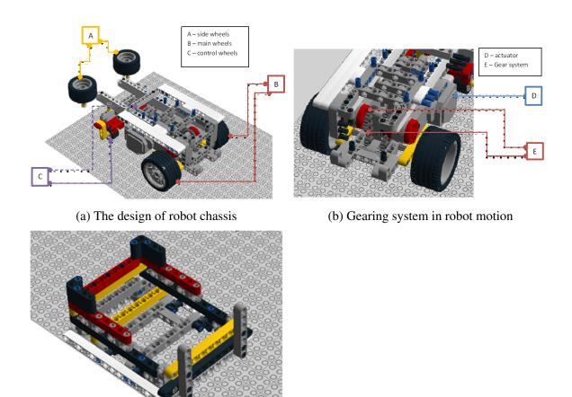
(c) Bracket design for holding SBC
