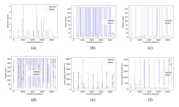
Fig. 3.6 The completed data after completing 1 voyage (8-meters) (a) ambient light, (b) color, (c) reflected light (d) lidar angle (e) lidar distance, (f) ultrasonic pulse
