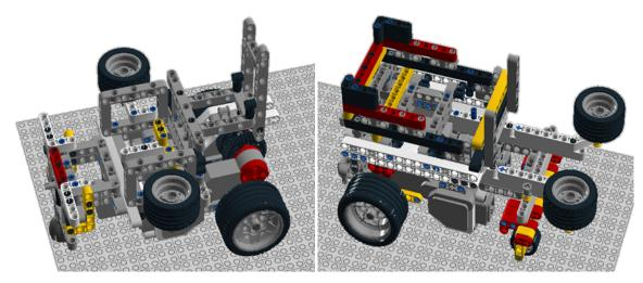
(a) First robot prototype with one control wheel(b) Final robot design using 2 balancing wheelFig. 3.2 Design of the proposed ILI with the decomposed structure of the robot components
