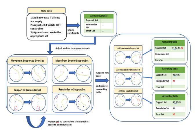
Fig. 3.4 The process of online SVM - the new cases is added after adjusting the observed vectors to the appropriate sets with respect to the constraints
