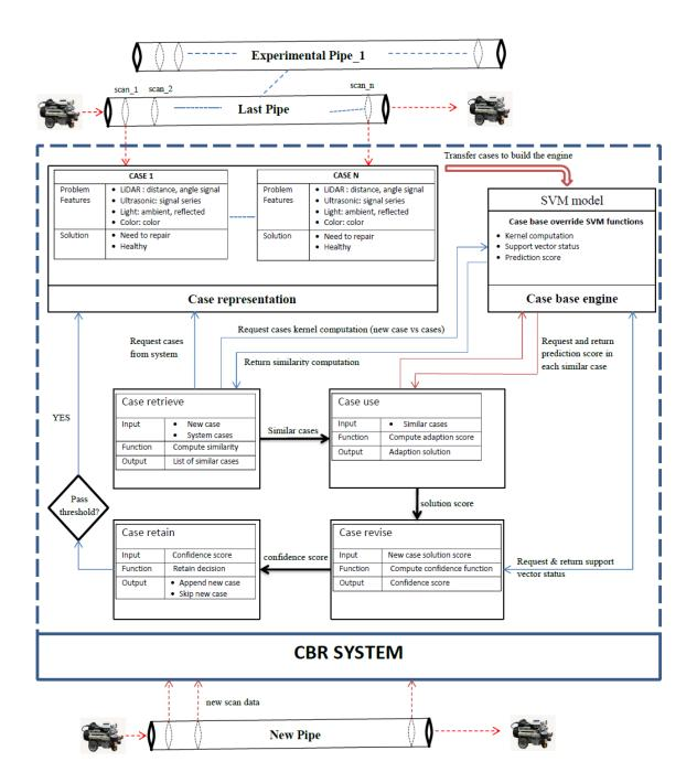
Fig. 3.8 The complete CBR diagram govern by online SVM for pipe defect detection system
