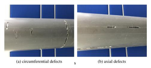
Fig. 3.5 Experimental defect pipe design for robot inspection mission
