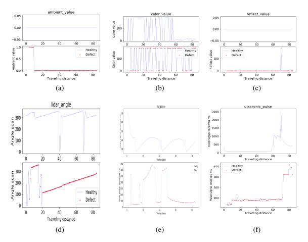
Fig. 3.7 comparison on healthy signal (upper) and defect signal (lower) in a small chunk of 8cm (a) ambient light, (b) color, (c) travelling light (d) lidar angle (e) lidar distance, (f) ultrasonic pulse
