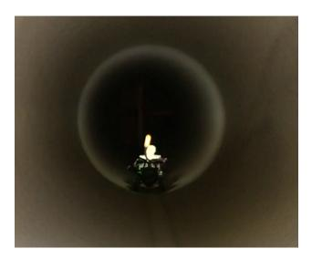
Fig. 4.2 The inspection gauge travels inside the pipe to transmit scanning signal for CBR system
