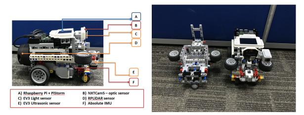
(a) The implementation of robot wielding all sen-(b) The implementation of the first prototype (left) sors and final design (right)
