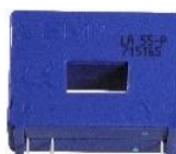
Fig. 8.10. Voltage sensor used to measure the battery voltage
