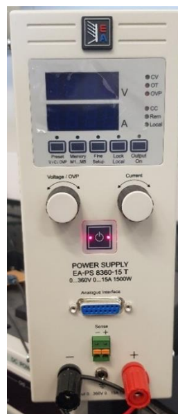
Fig. 8.2. DC power supply used to obtain a constant DC voltage on the Bus
