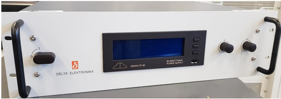
Fig. 8.6. DC\DC bi-directional supplier used to emulate the battery behaviour
