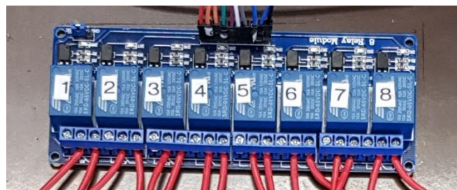
Fig. 8.4. Switches module board used to connect or disconnect a load from the DC Bus
