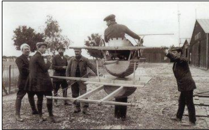
Fig 2-4 "Antoinette's Barrel", one of the earliest HIL simulator concepts from 1910s [36]
