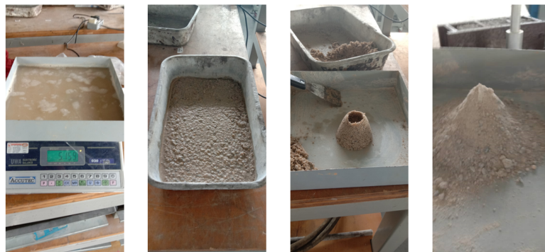
Figure 3.3.2: Testing aggregate for moisture conditions.
