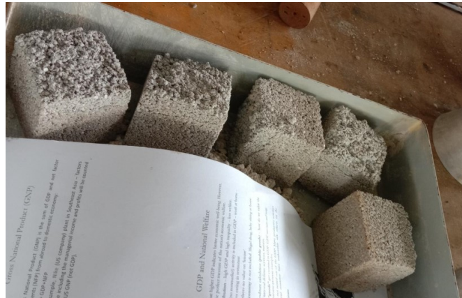
Figure 3.3.1: Failed mortar trial mixes.
