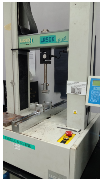
Figure 3.4.6: Illustration of set-up for flexural testing of small cement beams.
