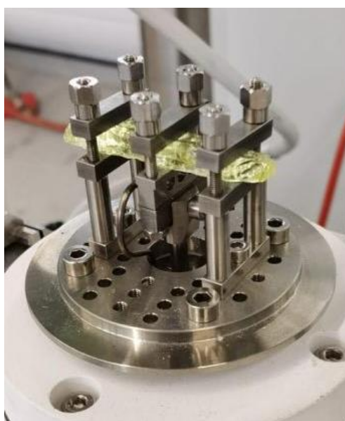
Figure 5.30 | Dual-cantilever programme for DMA analysis. Material on image: DBS- i Pr in PiBnA
