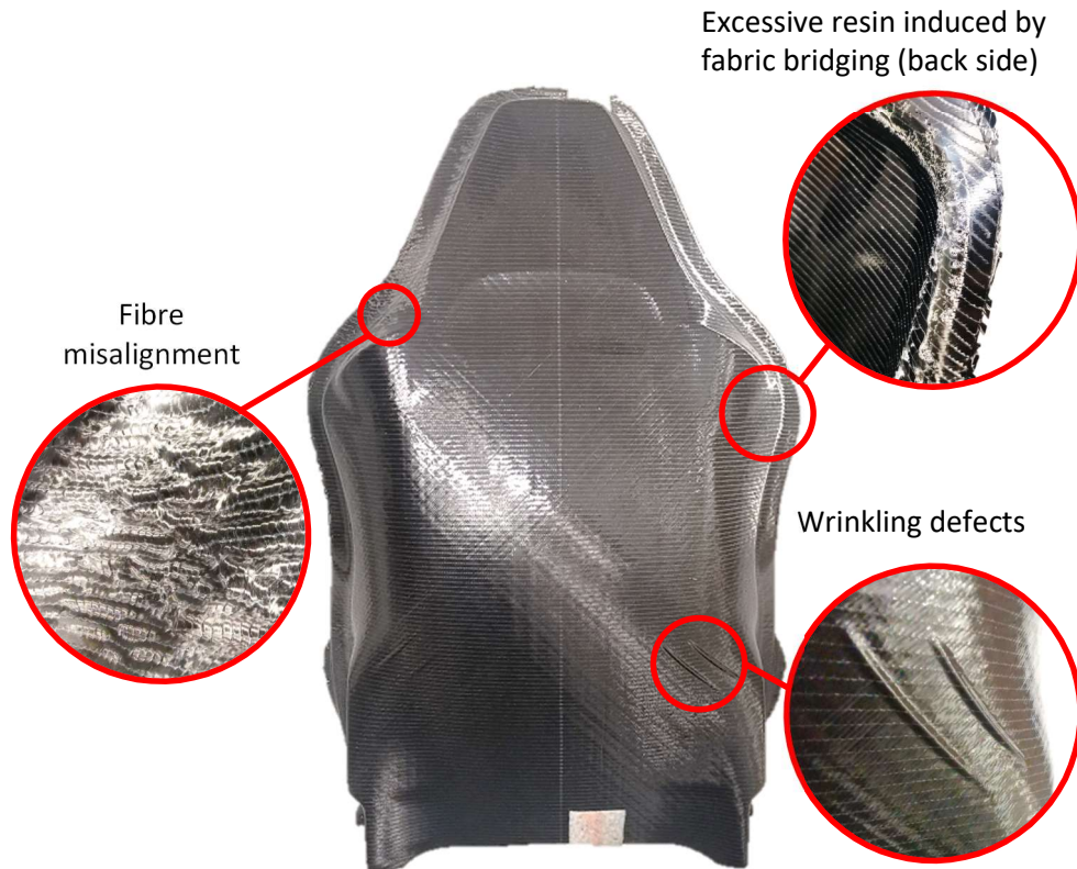
Figure 1.1 Typical modes of forming induced defects in a composite seat back.
