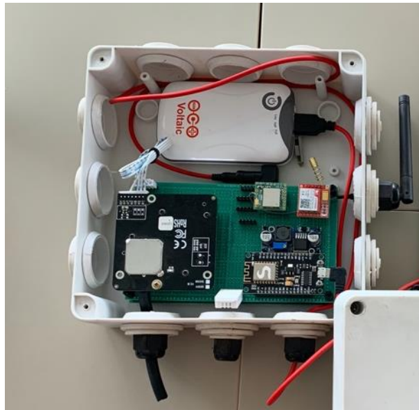
Figure 5-4: sensors.AFRICA's air quality sensor – internal components.
