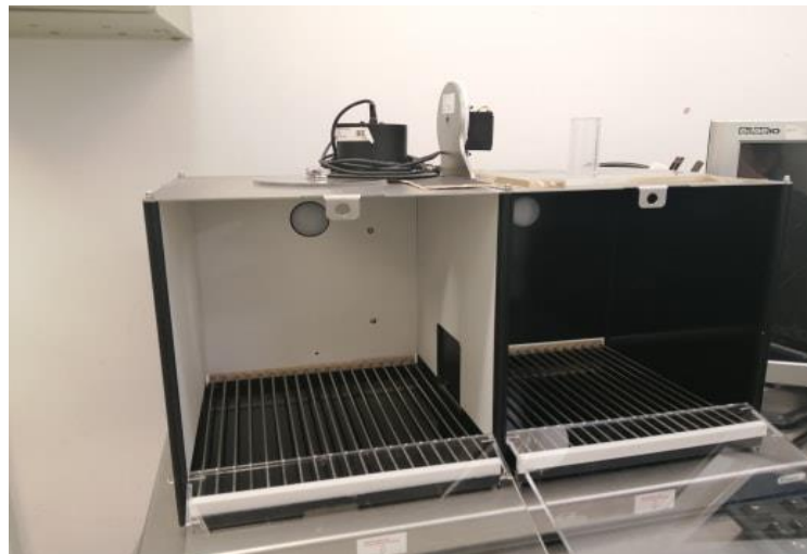
Figure 2.9 Two compartment box used to assess CFR.
