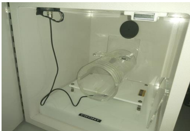
Figure 2.8 SR-lab startle response chamber used to assess PPI.
