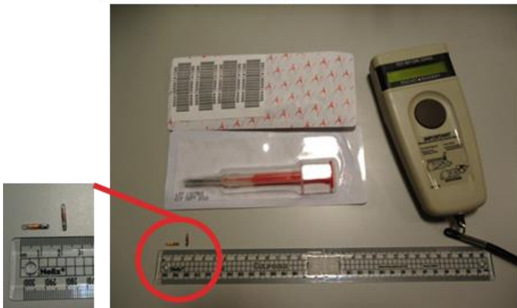
Figure 2.2 Microchip and scanner used to measure body temperature throughout experiment. On PND 27 – 31, adolescent male Lister hooded rats ( n = 40 ) received non-surgical subcutaneous implantation of a temperature-sensing microchip (Bio-
