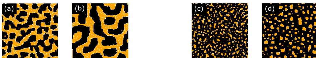
Figure 6.3.4: Examples of feature coarsening in the Rabani et al. 24 monte carlo model. For a ‘labyrinthine’ structure as generated with the parameters k_B T = 0.3 , \mu = 2.9 , MR = 3 , C = 0.4 , \epsilon_{nl} = 1.5 , \epsilon_{nl} = 2 , we observe visible coarsening from (a) 300 to (b) 1500 steps. By changing to k_B T = 0.32 , \mu = 3.2 , and C = 0.2 , we can generate an ‘island’ type image, and observe coarsening between (c) 100 and (d) 1000 steps.
