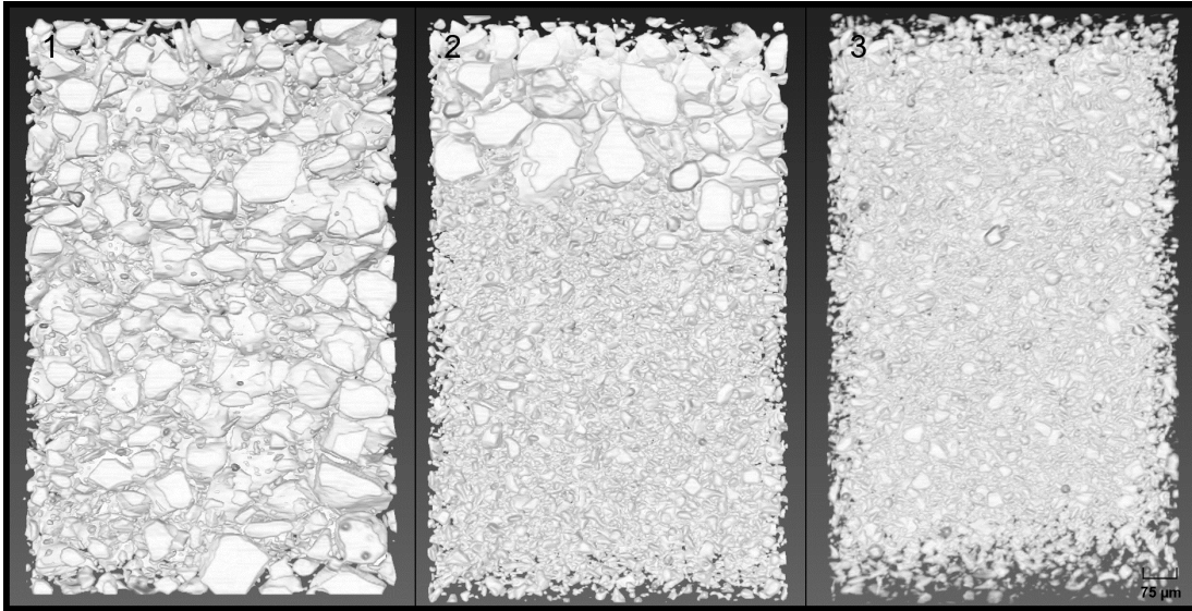
Figure 7.4: The three zones analysed in sample 12; zone 1 is composed of 75-180 \mu\text{m} grains, zone 2 is composed of 0-180 \mu\text{m} grains and zone 3 is composed of 0-75 \mu\text{m} grains.
