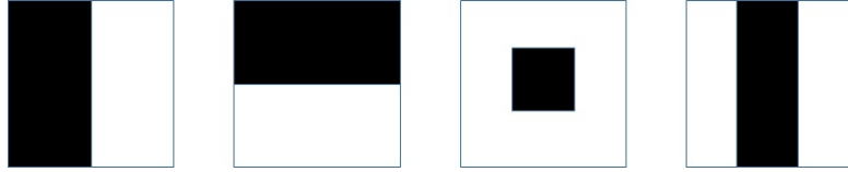
Figure 3.5: Examples of the Haar-like features used in the experiment
