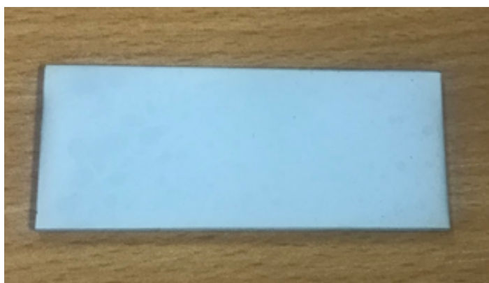
Figure 7.9: Ga_2O_3 and 45S5 co-sprayed coating deposited at 50 kW.
