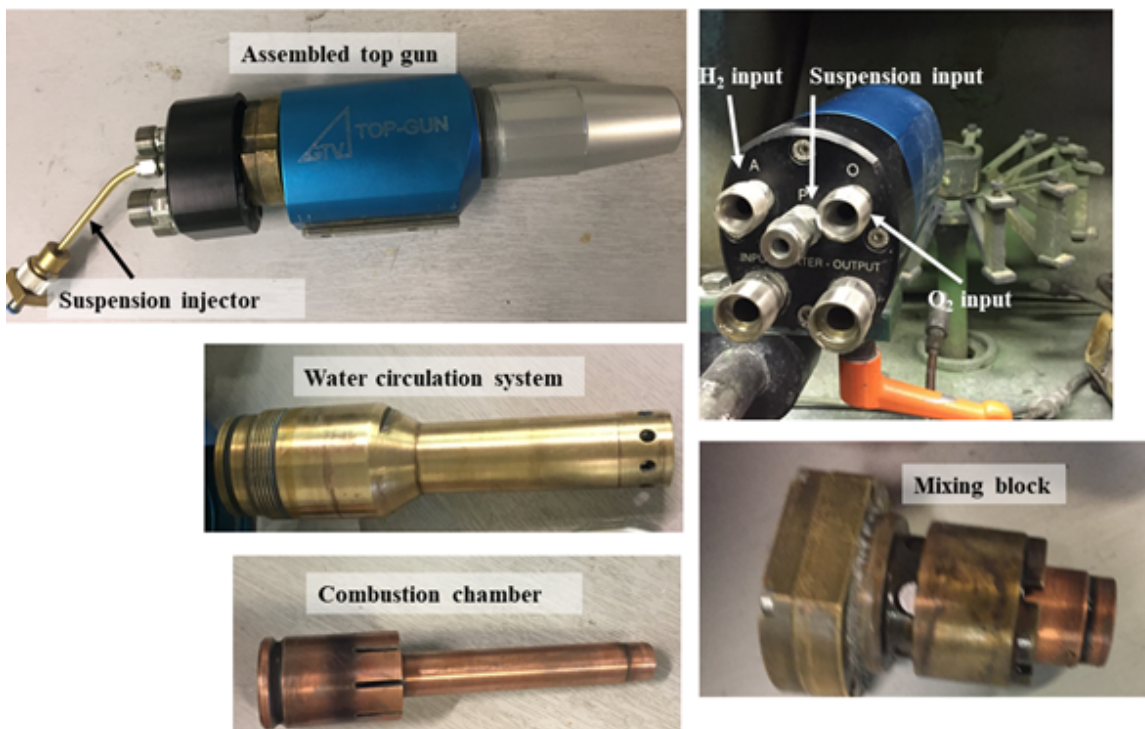
Figure 3.6: Different parts of UTP top gun for SHVOF spraying.
