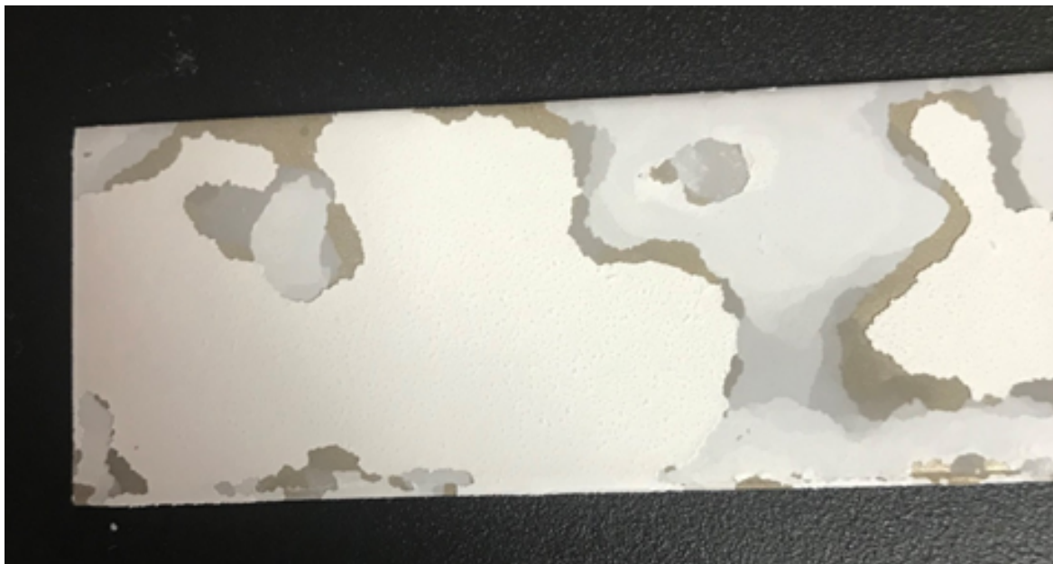
Figure 7.7: Ga_2O_3 doped Bioglass ® coating deposited at 50 kW.
