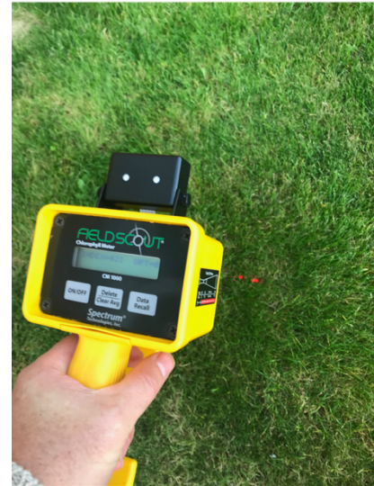
Fig 18. Using the Field Scout CM1000 Chlorophyll Meter. (From author's library)
