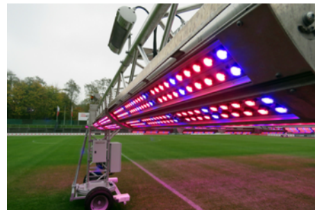
Fig 5. LED lighting showing the red and blue wavelengths. (Photo taken on a visit to present to groundstaff.)
