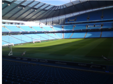
Fig 2. The Etihad Stadium, Manchester City FC, illustrating how the high stadia construction reduces direct light to the playing surface. From the author's private collection.
