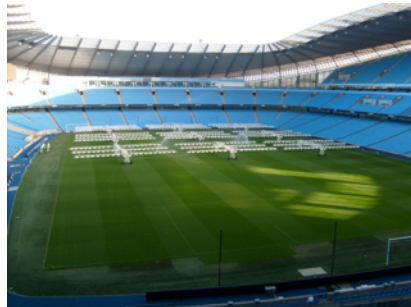
Fig 4. High Pressure Sodium lighting rigs at The Etihad Stadium, Manchester City FC. (Photo taken on a visit to present to Premier League groundstaff.)
