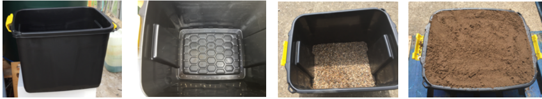
Fig 9. L-R: The plastic container selected for the trial, holes drilled in the base, layer of 6mm grit consolidated rootzone
