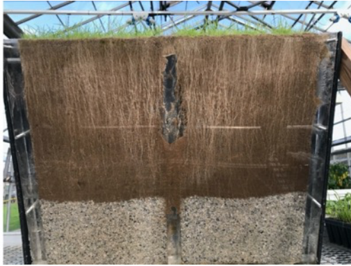
Fig 10. USGA rootzone overlying gravel showing turfgrass roots ( Lolium perenne spp. L.) and demonstrating a perched water table, with saturated zone near the gravel and drier rootzone (air entry) near the surface. Taken on 28 th Oct 2019 at The University of Nottingham - Sutton Bonington Campus, Sutton Bonington, England. From the author's private collection.)
