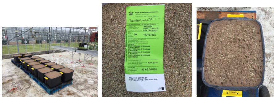
Fig 11. L-R: Containers filled with rootzone, list of cultivars of L.perenne L. in the blend, seeded container.
