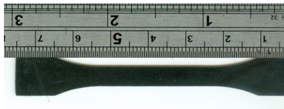
Figure A.2: A dumbbell shaped specimen cut for uniaxial tensile testing. The image was scanned using a HP Scanjet G4010 scanner at 1200 dpi.
