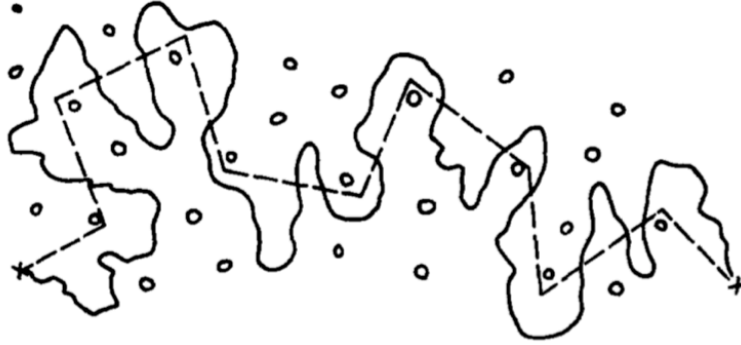
Figure 2.14: An illustration of the tube model concept. Entanglements form the tube and the centre of the tube is represented as dashed lines. The solid line represents a polymer chain that has been cross-linked at its ends. The hollow circles represent other polymer chains that are perpendicular to the surface of the tube. Adapted from [80].
