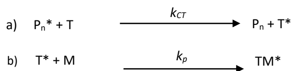
Scheme 1-4. Representation of the chain transfer mechanism for a typical CTA.
