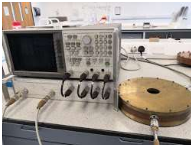
Figure 3.13 Benchtop measurement system of a cylindrical resonant cavity
