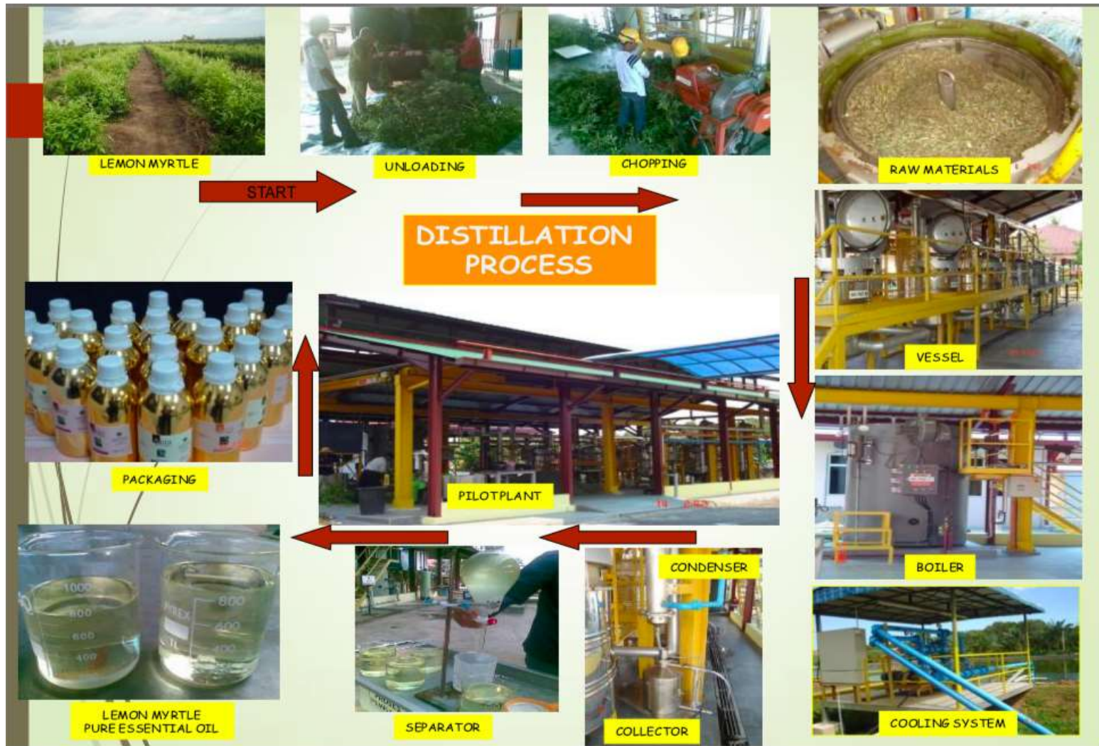
Figure 2.1 Industrial distillation process to produce Lemon Myrtle essential oil (Source: Bakri, 2015)
