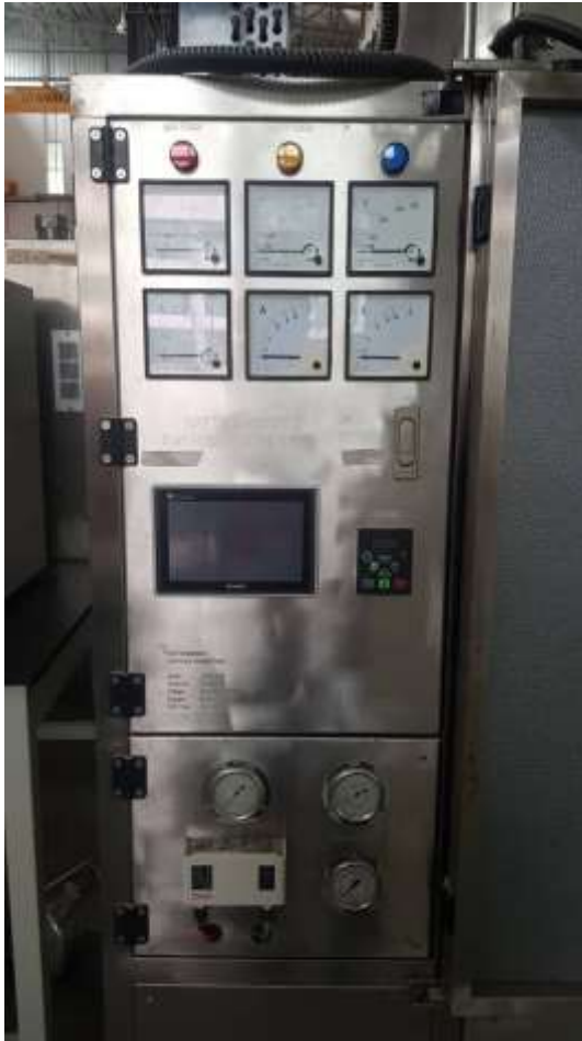
Figure B1 Control panel for Heat pump dryer
