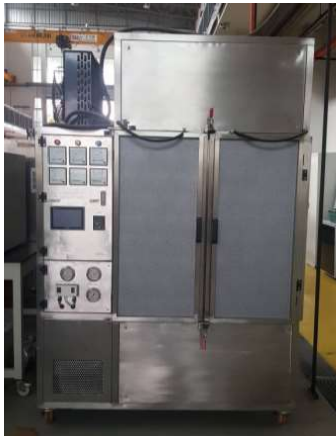
Figure 3.3 Heat pump dryer unit
