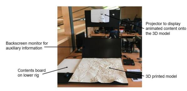
Figure 12. Annotated PARM display rig.
