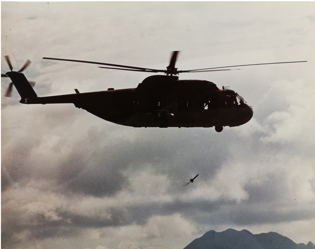
Figure 5.1: Photograph caption: 'Side view of an CH-3E helicopter dropping an ADSID (Air Delivered Seismic Detection Sensor) sensor over Laos' (Gaston 1968).
