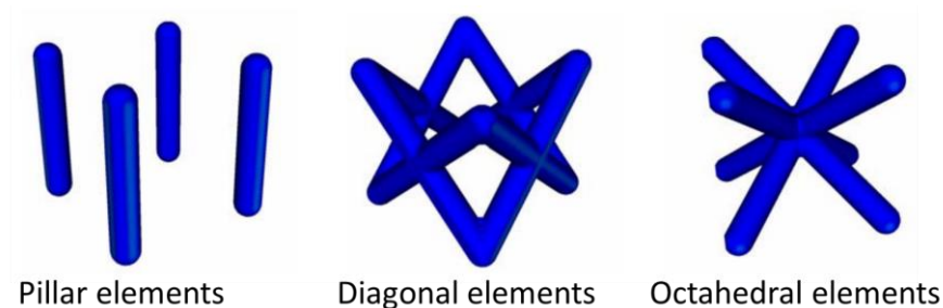
Figure 2.10. Types of elements that can be produced by the software of Brooks et al. [48]
