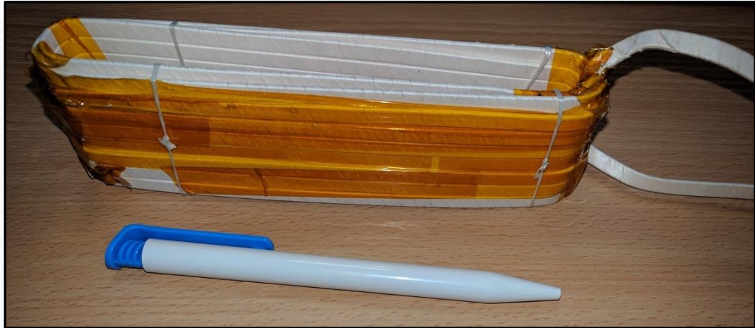
Figure 4-1: Example of a traditional tightly wound copper coil made from rectangular cross-sectional wire with paper and Kapton tape insulation (Provided by the Power Electronics, Machines and Control Research Group at the University of Nottingham).
