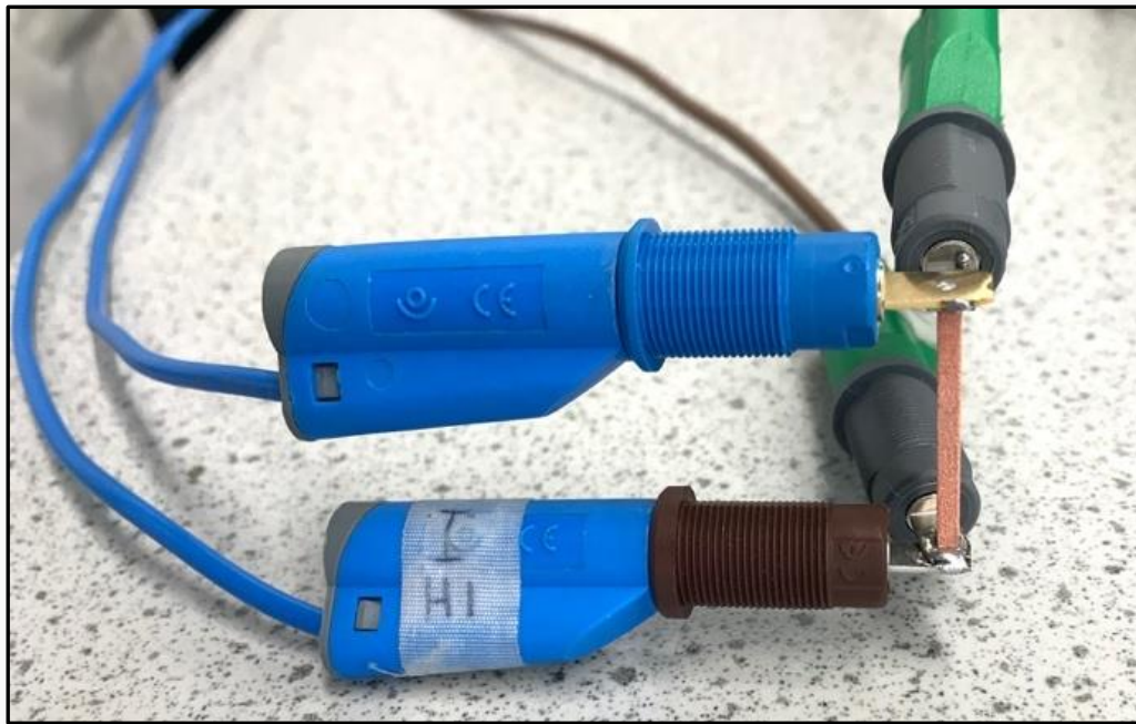
Figure 3-17: Copper test specimen soldered directly to electrical tabs in order to minimise contact resistance as measured by a 4-point probe.
