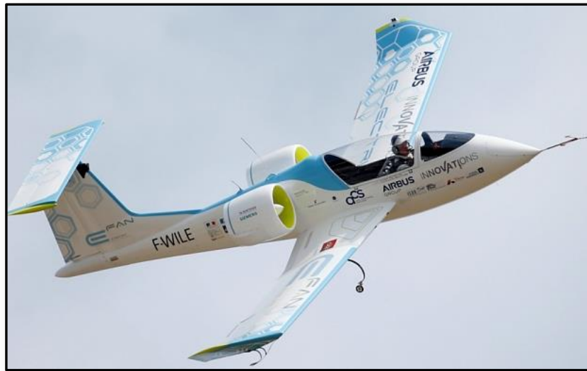
Figure 2-14: The Airbus E-Fan personal all-electric aircraft AEA at the Paris Air show in 2015 [100].
