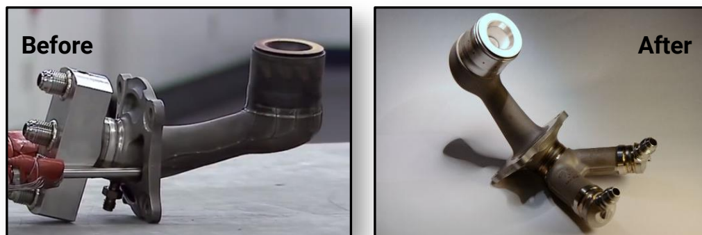
Figure 1-4: DfAM level three – Combine multiple parts as with the GE Leap fuel nozzle before redesign [41] (right) and after redesign [42] (left).
