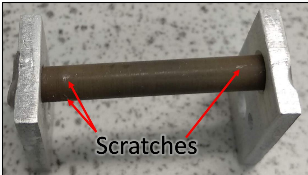
Figure 0-4: After testing the insulative ability of the anodised AlSi10Mg, scratches appeared on the surface.
