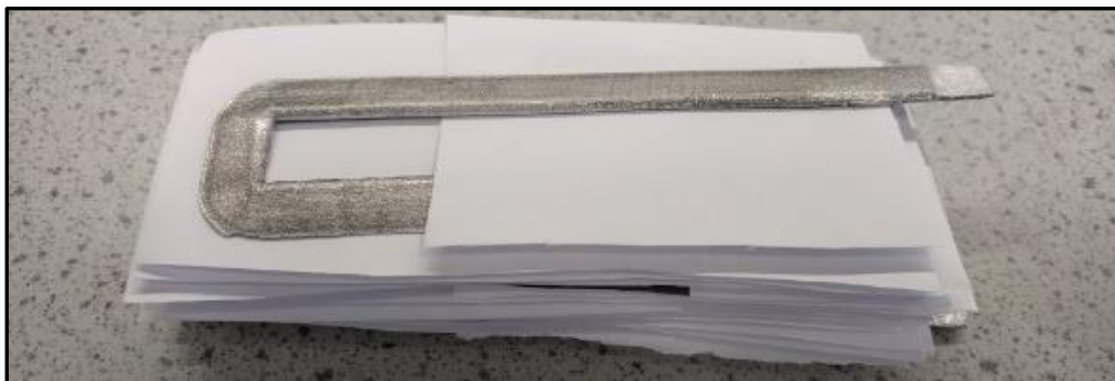
Figure 6-10: Paper insulation used for electrical testing of 3D printed electrical coil.
