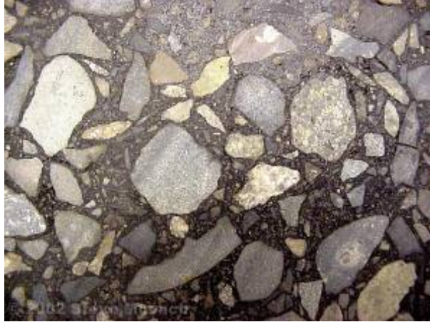
Figure 2-3 Dense-graded HMA (Pavement_Intracative, 2010)
