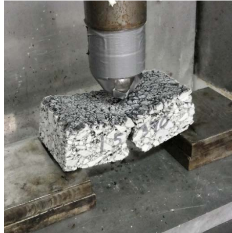
Figure 3-4 Prismatic test specimen and 3-point bending test
