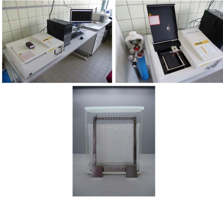
Figure 3-8 TLC-FID Iatroskan® equipment used at BRRC laboratories.
