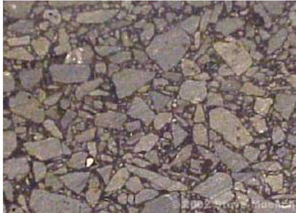
Figure 2-4 Gap-graded HMA (Pavement_Intractive, 2010)
