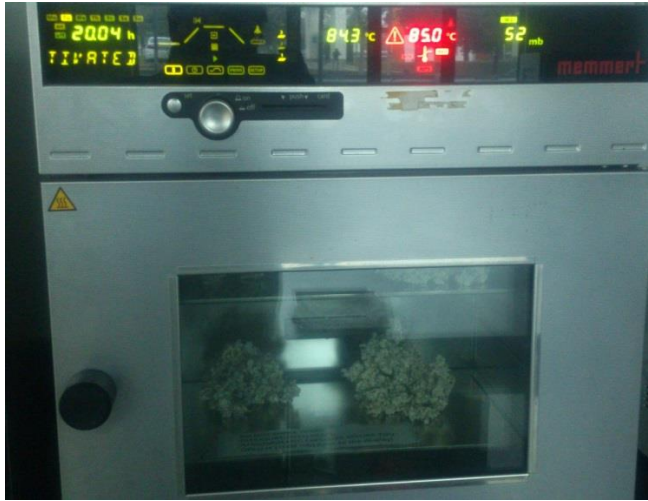
Figure 3.8: Laboratory scale vacuum dryer
