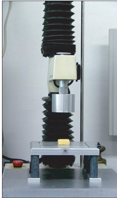
Figure 3.11: Texture analyser for texture measurement
