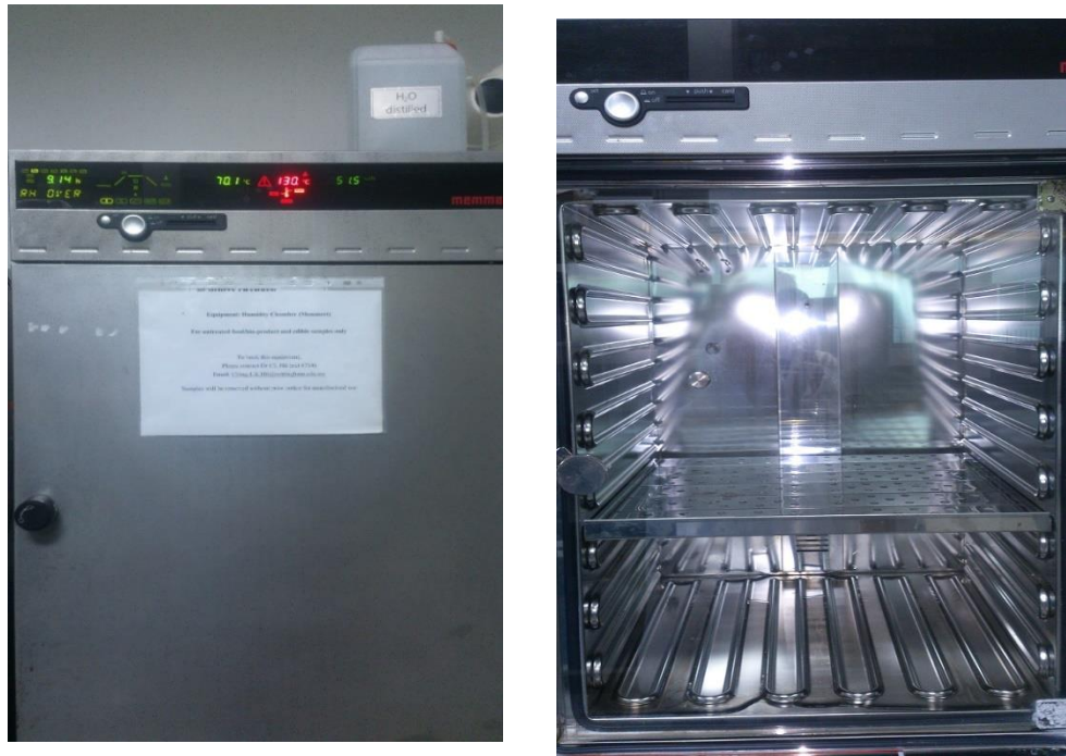
Figure 3.7: Laboratory scale hot air convective dryer
