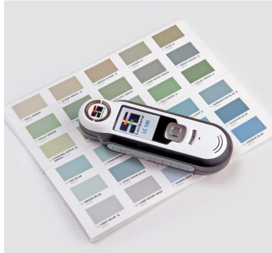
Figure 3.10: Lovibond LC100 for colour measurement
