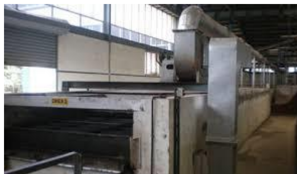
Figure 1.7: Tunnel dryer for crumb rubber
