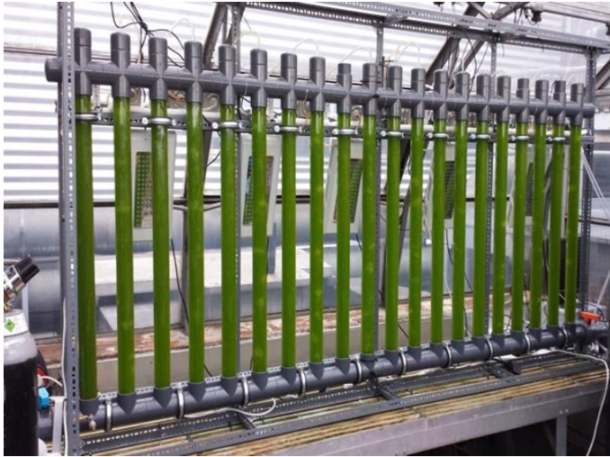
Figure 6: Picture (Variconagua,2016) and schematic diagram of an airlift photo bioreactor
