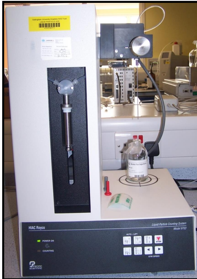
Figure 3-3 HIAC 9703 apparatus used in quality control unit to quantify the particles' size
