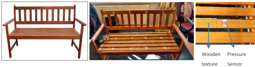
Figure 177 - Left: Garden Bench, Centre: Sensors location, Right: wooden texture used to hide the sensors
