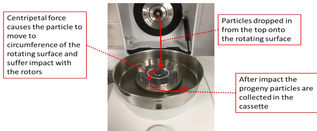
Figure 8.1 displays a Retsch ZM200 mill, set up with no screen so that particles when passed through experience only 1 impact before size analysis is completed.
