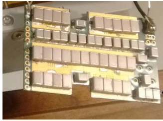
Figure 4.21- The output Capacitor C_o ( 4 \mu F ).
