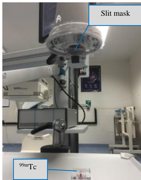
Figure 3.2: Photograph of experiment set up during intrinsic spatial resolution test. A ^{99m}\text{Tc} point source was positioned at a distance of 250mm from the attached slit mask.
