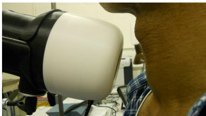
Figure 8.3: Photograph of the head of the HGC which was mounted on an articulated arm during imaging of the patient neck area.
