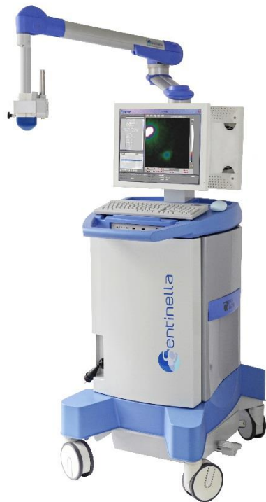
Figure 1.14: SFOV gamma camera mounted on an articulated arm and cart based system (left) with pinhole collimator, Sentinella 102 (image courtesy of Victoria García, OncoVision, Spain) and (right) MGC 500 with parallel-hole collimator (Taken from [54]).
