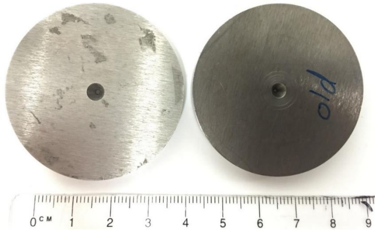
Figure 2.11: Bespoke pinhole collimator for HGC with pinhole diameters of 1 mm (left) or 0.5 mm (right).
