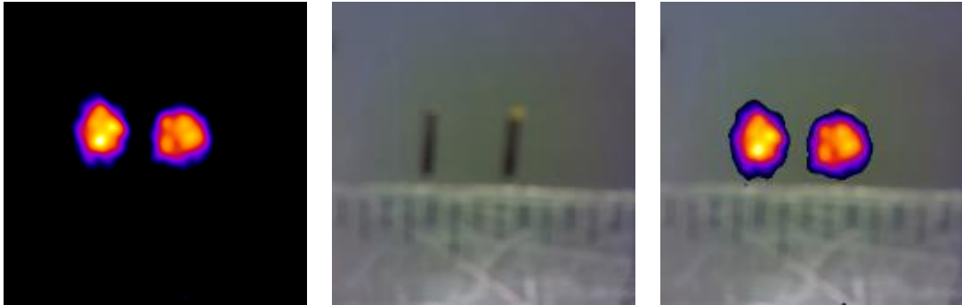
Figure 5.19: Gamma (left), optical (middle) and hybrid (right) images of the ^{125}\text{I} seeds placed with a separation distance of 3 mm, taken by Nebuleye mounted with 1 mm diameter pinhole collimator with SCD of 30 mm and 10 minutes acquisition time.
