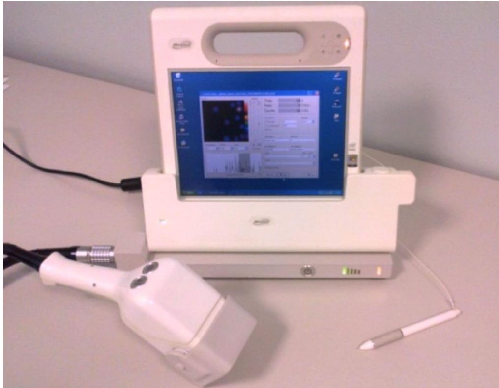
Figure 1.12: Example of SFOV gamma camera with CsI(Tl) scintillation detector coupled to PSPMT (IP Guardian2, Li-Tech, Roma, Italy). Photograph courtesy of Domenico Rubello, MD, Rovigo, Italy.
