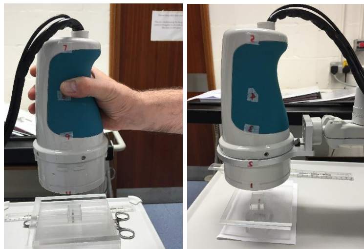
Figure 7.2: Operator hand movement study set up. Point source was placed underneath of the camera head held by an operator (left) with extended right hand or mounted on an articulated arm (right) at a SCD of approximately 7 cm.
