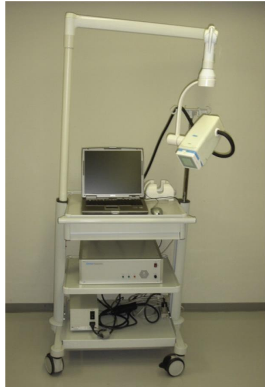
Figure 1.14: SFOV gamma camera mounted on an articulated arm and cart based system (left) with pinhole collimator, Sentinella 102 (image courtesy of Victoria García, OncoVision, Spain) and (right) MGC 500 with parallel-hole collimator (Taken from [54]).
