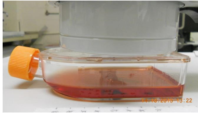
Figure 6.6: Experimental set up of the system uniformity and sensitivity tests. The camera head was positioned above the flask containing the flood source (mixture of ^{99m}\text{Tc} solution and red coloured dye).
