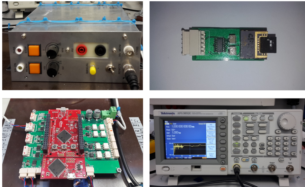
Figure A.2: Power converter (top left), MEMS-based cantilever sensor (top right), XMC4500 Relax Kit (bottom left) and AFG3000 (bottom right).
