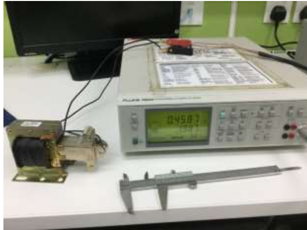
Fig A. 3 Measurement device for the inductance graph.
