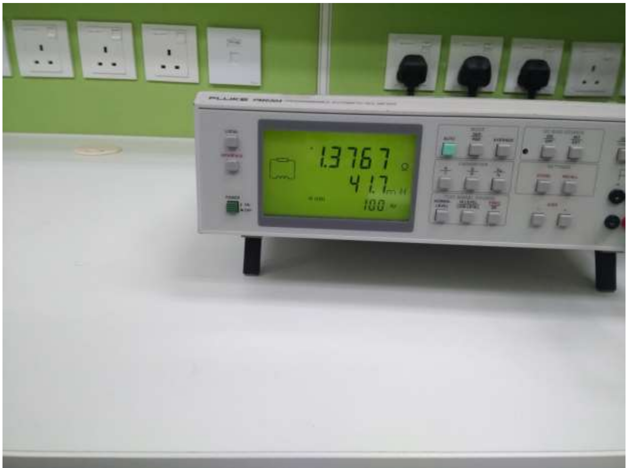
Fig A. 4 The resistance and inductance is displayed when connected to the solenoid.
