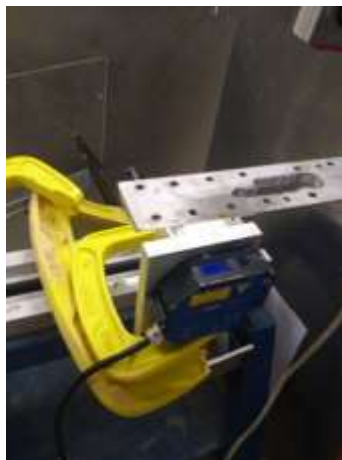
Fig 3.10 Laser sensor was clamped to a stationary object.
