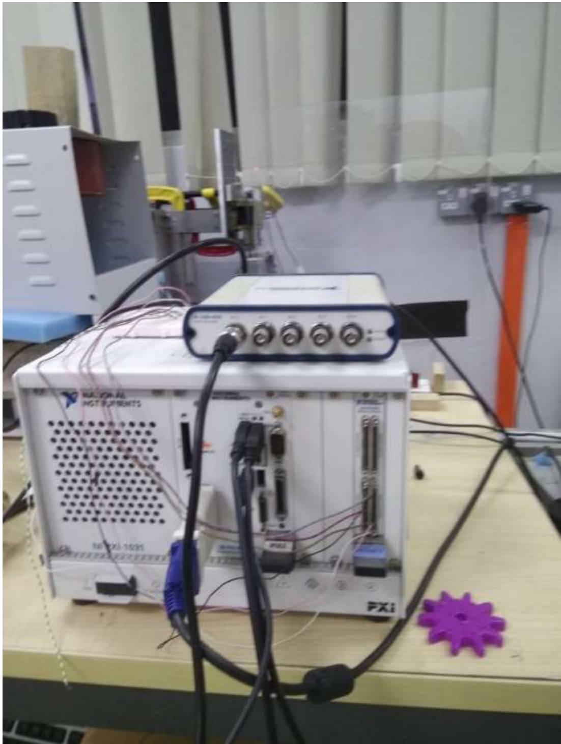
Fig A. 5 PXI connected to the NI USB 4432 to get the result from the motor
