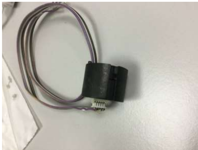
Fig 3.8 (a) connection of the cables to the Arduino and (b) housing and the picoblade suitable for the magnetic encoder.
