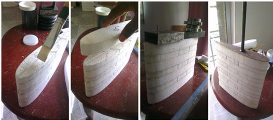
Figure 5.37: Bonding Process of MTS with spanwise patterned slots.
