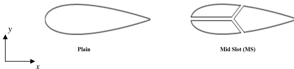
Figure 4.1: 2D Section of Plane and Mid slot (MS) NACA0018 aerofoils.
