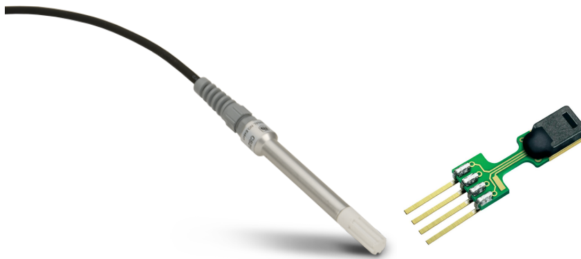
Figure 3.2.6: Pictures of the Temperature and Relative Humidity probe and its digital sensor, [6]
