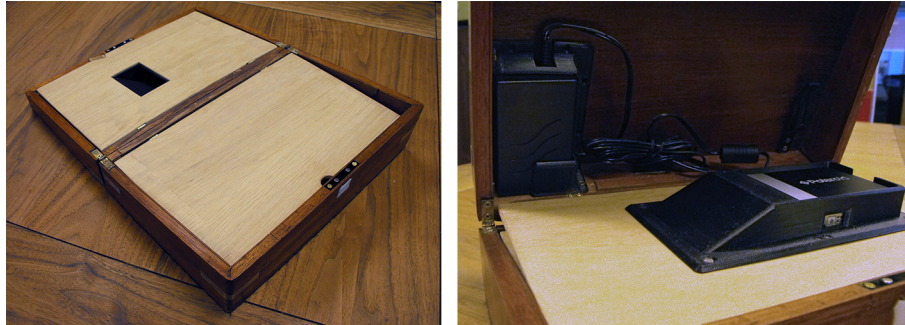
Figure 9: The new interior panels [Left]. The small photo printer hidden in the lid of the box [Right]
