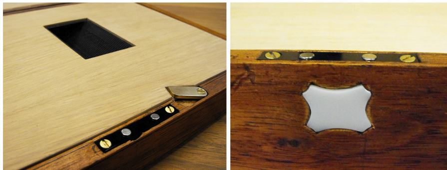
Figure 10: The magnetic connections in the lid and base of Photobox mean that it can only print when closed. These also connect the printers 'out of paper' light.
