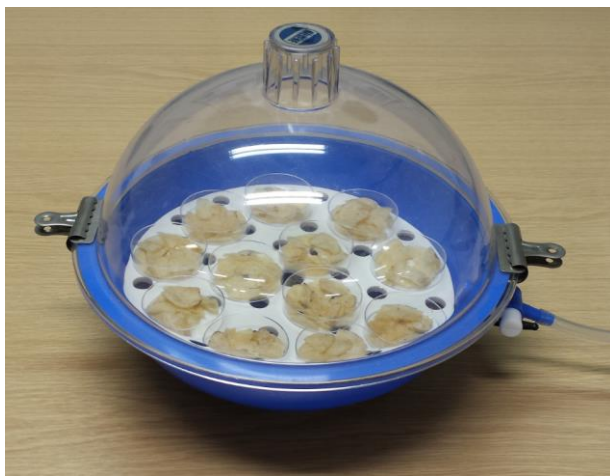
Figure 4-9 Desiccator loaded with sample dishes for dehydration using dry nitrogen
