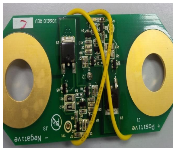
Figure 3-9: (a) & (b): Voltage equalization circuit 1 (for 2 & 5 SCs); (c): Voltage equalization circuit 2
