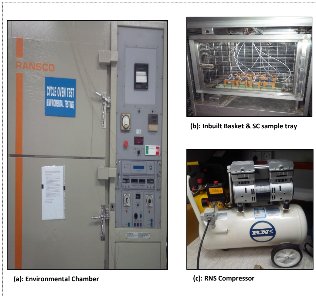
Figure 3-6: (a): Ransco environmental chamber; (b): SC sample tray placed inside the chamber; (c): RNS cooling compressor
