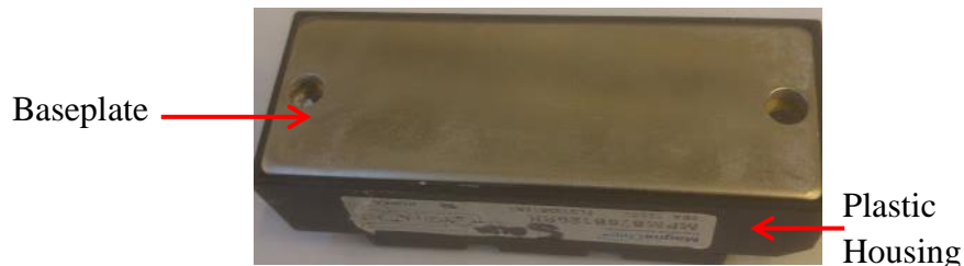
Fig 2.6 : Baseplate of an IGBT module & plastic housing
