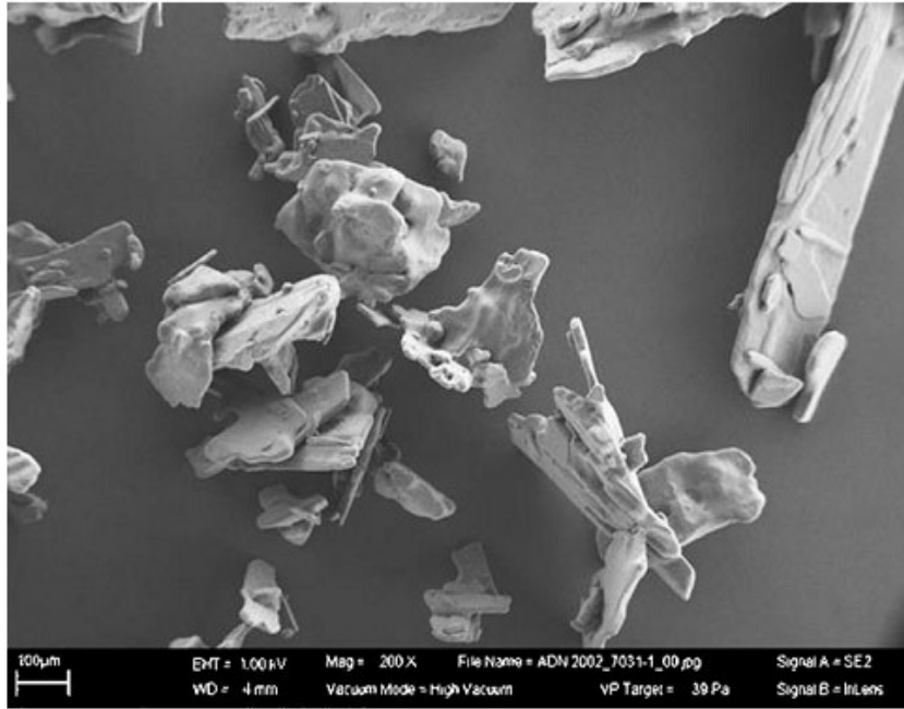
Figure 4-19 SEM image of ADN (Heintz, et al., 2009) showing needle like structure.
