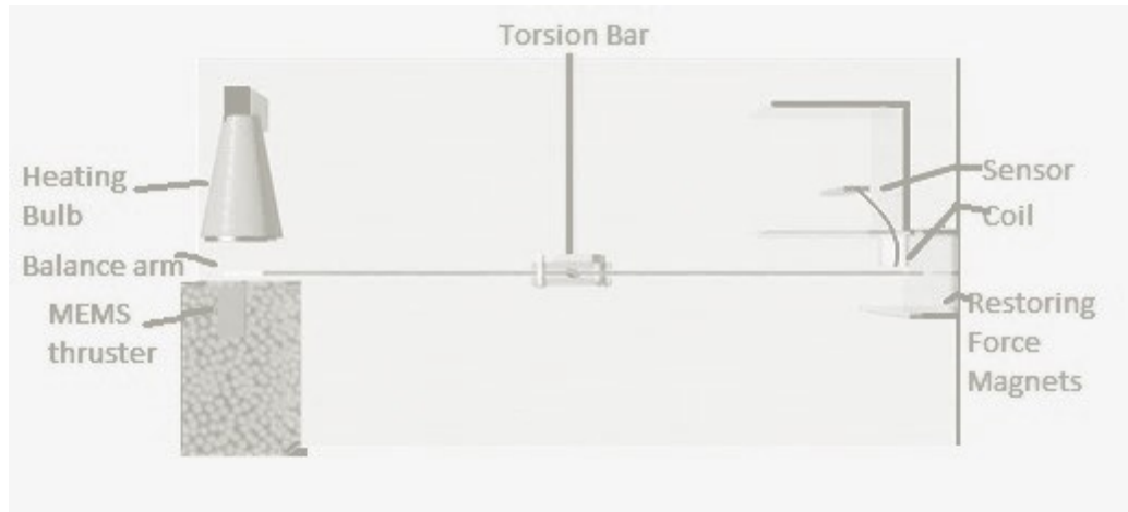
Figure 5-8 AutoCAD generated Top view of the thrust measurement system
