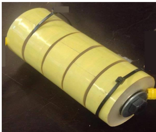
Figure 7.16 the photograph of the resonant capacitor
