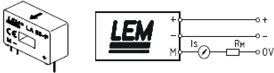
Figure 7.14 the LEM-LA 55-P transducer and its connection diagram
