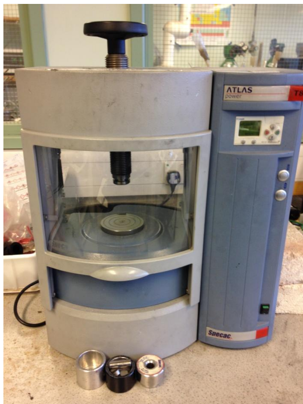
Figure 3.10 –Specac Ltd. T8 hydraulic press, die and moulds used for pellet synthesis from oxide powders.
