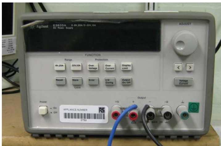
Figure 3.13 - Agilent E3633A 20A/10V Autoranging DC power supply.
