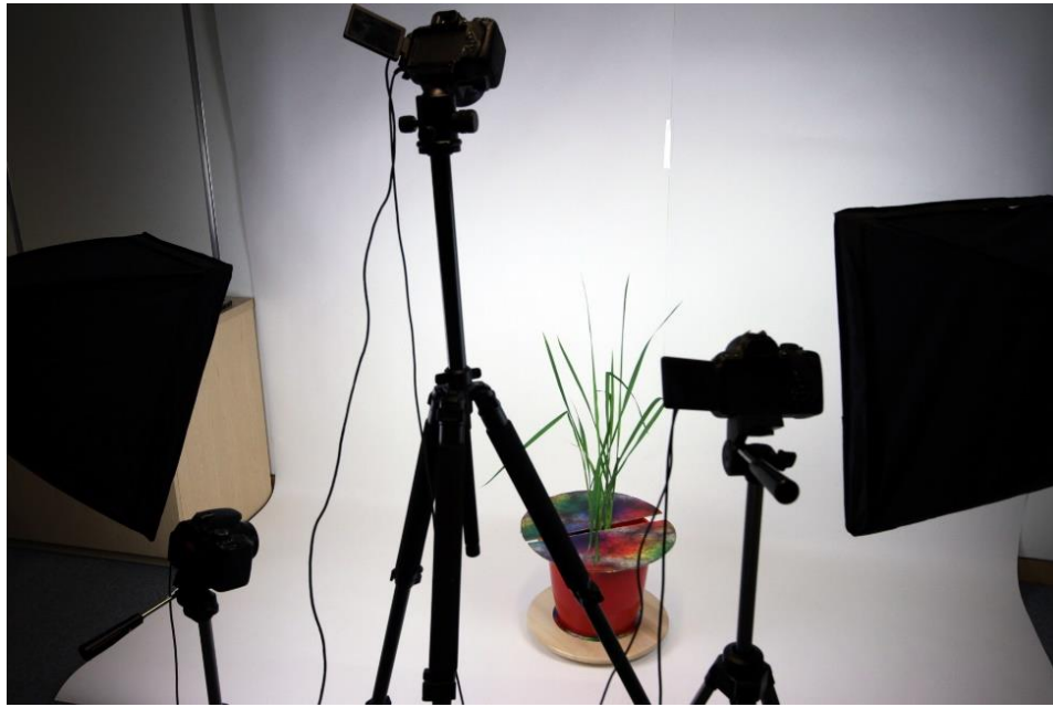
Figure 2.2: Set up of the imaging studio for single plant imaging. Plants are imaged using 3 fixed Canon 650D cameras on tripods. A turntable enables the plant to easily be rotated whilst a calibration target (coloured cardboard) aids the process and is of a fixed size, to allow the reconstructions to be scaled back to the original units. Supplementary lighting is provided if necessary.
